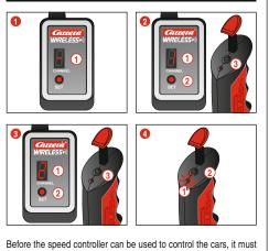
be "bound" to the receiver. To do this, switch on the control unit.
