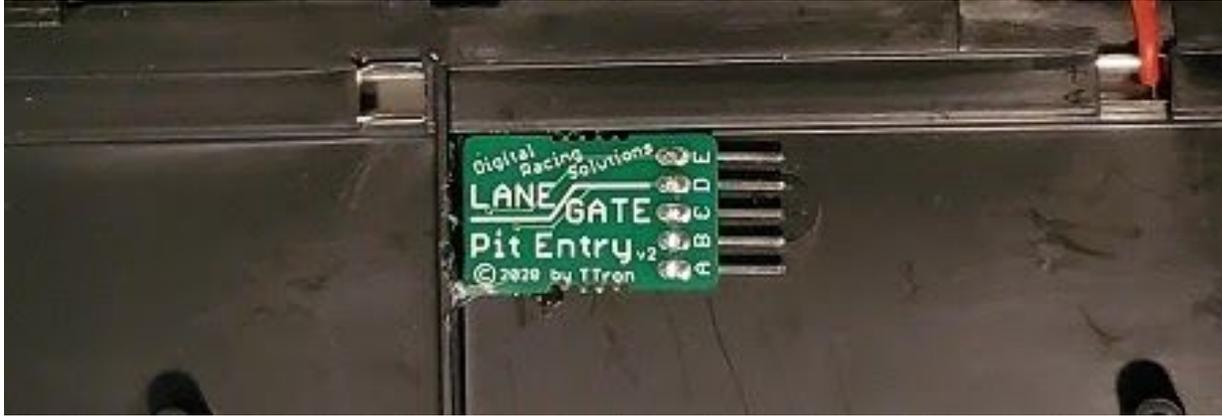
5. Locate the red wire shown below and gently pull its spring clip out of the track rail. Cut off the clip, then use wire strippers to remove 4mm of insulation from the end of the wire.
