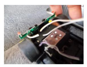
STEP 3: Set aside the quick connect wire and remove rear light board by pulling it up out of car.
