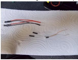
STEP 5: Use caution and strip the wires on the quick connect about ¼ inch and attach the quick connect to the new LED Lights making sure you connect the Yellow wire on the quick connect to the Red wire of the new Led lights, cross wires as if making an "X" and then twist tightly, bend your twist back straight and then slide the two pcs of heat shrink tubing over the connections and heat until it has shrunk (You can use a lighter if a heat gun is not available)
