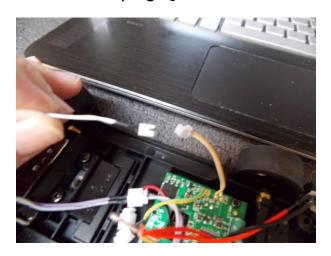
STEP 2: Cut wire as close to Rear Board as possible.
