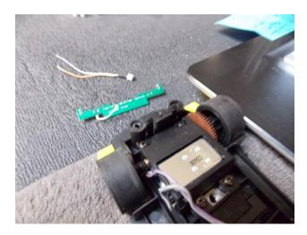
STEP 4: Remove the rear tail lights from the bag along with the 2 pcs of heat shrink tubing and locate the quick connect you cut off in step 2.
