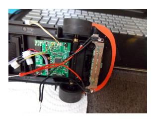
This is the final step. Make sure all adhesive or glue has hardened and that all of your quick connects are back together. Make sure your wires are tucked inside of the car close to the body where they will not be pinched. Put the body back on the car and tighten your chassis screws.
