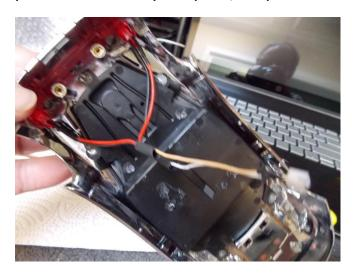
STEP 7: Locate the front headlight board, unplug the quick connect wire from main board. Next cut the wires off of the light board (as close as possible to the board). Next look at the front board and you will see two little bulbs, bend them back and forth until they break off and the board is now clean. Remove your new Led lights from the package, you will see that they are bent in a way to get around the wheels (If you need to bend them a little more you can do so)
