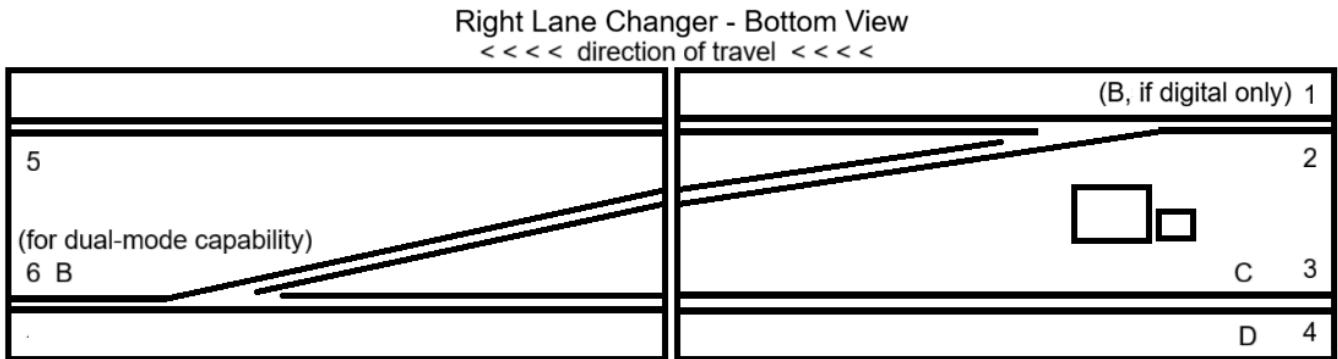
Wire B must be extended and connected to rail #6 in the exit section.
