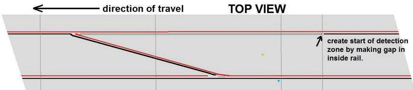
16. Creating the isolated rails means the track rails are no longer a continuous loop, so power taps/jumpers may need to be added. Choose their location carefully. Do not place a power tap on the isolated rails inside of the detection zone.
