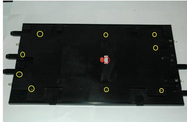
7. Place the section so that the IR sensor (with blue/yellow wires) is at top right. The numbers on the right side of the picture help identify each of the track rails. The factory black (-) wire may be located rail #2 or #4 and either position is acceptable. The factory red (+) wire must go to rail #1. If in rail #3 as shown below, move it to rail #1.
