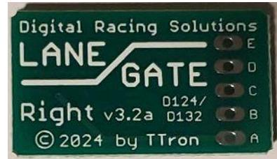
The DRS Lane Gate “Right” chip is for D124/D132 lane changers where cars can move from the left lane to the right lane only. That includes models #30345 Straight Type, #30362 Left Curve - In to Out, and #30365 Right Curve - Out to In
